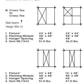
Cross tees tested as follows: ML7343 tested at 9.00 lbs./LF to 1/360 of 4' span.
